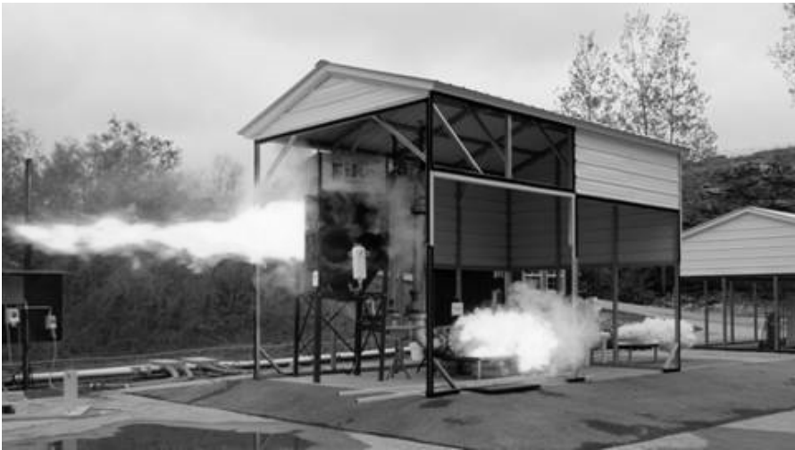
Figure 5.20. Dust collector explosion venting, courtesy Fike.
