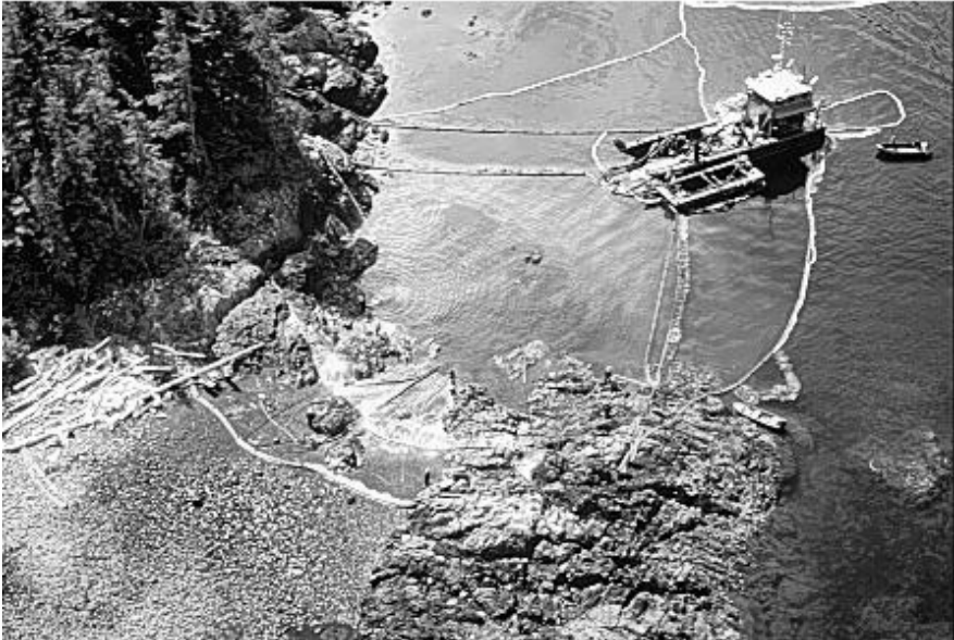
Figure 3.31. Aerial of a maxi-barge with water tanks and spill works hosing a beach, Prince William Sound, courtesy of Exxon Valdez Oil Spill Trustee Council.
